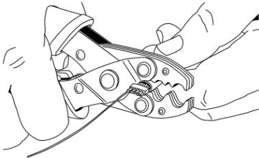
**4** Carefully insert into backend of connector (A) and push all the way forward (B) until all 8 conductors are seated flush against the front end.
