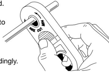
**2** Line up your wires and make a clean cut across all 8 conductors and slide on the wire guide bar.
