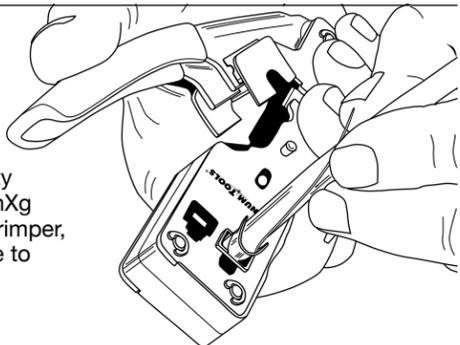
**6** Roll up the drain wire and place in the base of the external ground. As you start to bring the external ground into place onto the cable, keep the mass of drain wire tucked in so it is totally covered.
