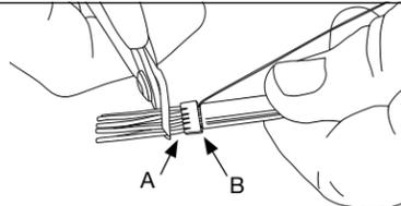
**3** Reshape the end of the cable using the CT-360 (PN 12360), making it oval so it slides into the connector with ease.
