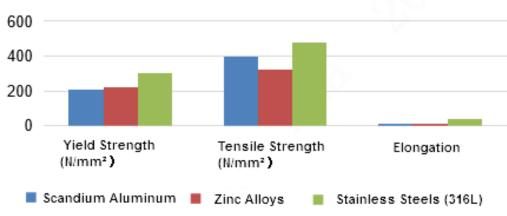
Figure 3.5 Tensile test performance parameters for different materials
