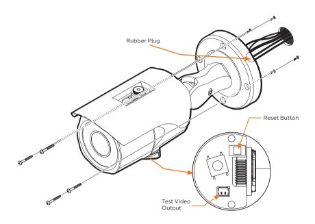
NOTE: Based on the installation environment, remove the rubber plug on the side of the camera's bracket and use the gap as a cable guide to prevent cables from getting caught between the camera and the mounting surface, which can cause damage to the cables or prevent a proper mounting.
