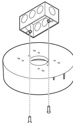
**NOTE:** When mounting the junction box to a gang box using installation option B, use the wall anchors and screws to secure the junction box and gang box to the mounting surface.
