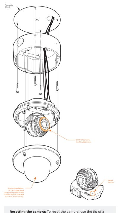
paper clip or a pencil and press the reset button. Pressing the button for five (5) seconds will initiate a camera-wide reset of all the settings, including network settings.
