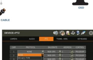
Camera type will be auto-detected and displayed under the camera tab. Protocol should match the camera type detected.
