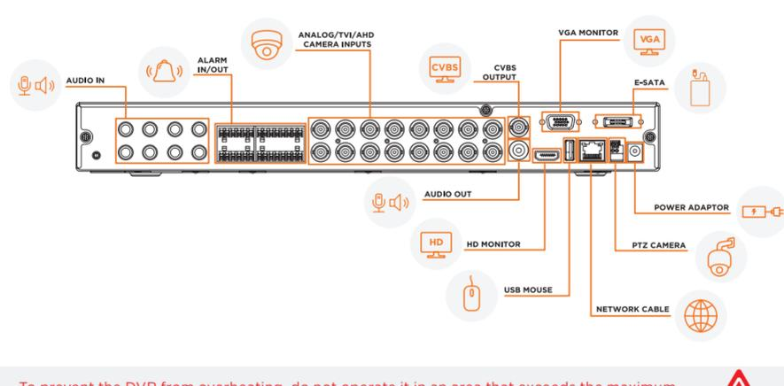
To prevent the DVR from overheating, do not operate it in an area that exceeds the maximum recommended ambient temperature of 104°F (40°C). To prevent airflow restriction, allow at least 3 inches (7.6 cm) of clearance around the ventilation openings.
