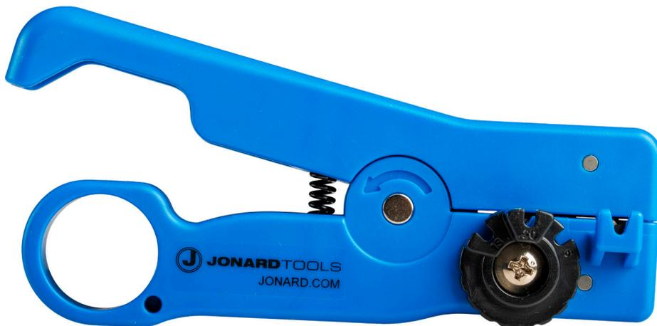
The EZSR-23 Fiber Slit & Ring Tool has been specially designed to prepare 2 mm and 3 mm fiber optic cables for connecting with Fitel EZ!Fuse™ SC & LC Splice-On Connectors. This tool saves time and makes the connecting process extremely easy by having a ringing dial and slitting channel with preset lengths. This slit and ring tool also features the following:
