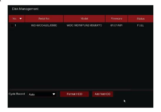
If the HDD is installed in the DVR for the first time, it must be formatted. Select the HDD and then click button Format HDD to format the HDD.
