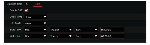
DST: Enable if Daylight Saving Time (DST) is observed in your region
