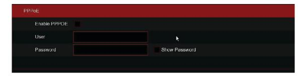
This is an advanced protocol that allows the DVR to connect to the network more directly via DSL modem.
