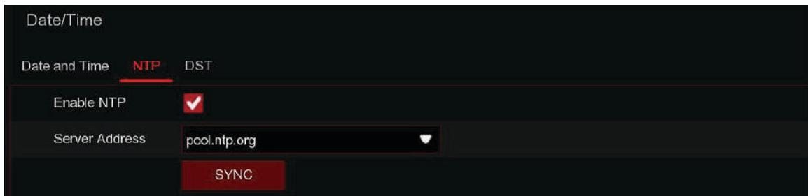
The screenshot shows a configuration menu titled "Date/Time". Under the "Date and Time" section, there are two tabs: "NTP" (which is selected and highlighted in red) and "DST". Below the tabs, there is a checkbox labeled "Enable NTP" which is checked. Underneath, there is a dropdown menu for "Server Address" with "pool.ntp.org" selected. At the bottom of the configuration area, there is a red button labeled "SYNC".
