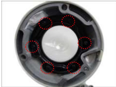
3. Remove the bracket and then the transparent dome cover.
