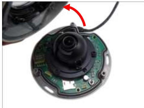
**NOTE:** A desiccant bag is attached underneath the dome cover. DO NOT remove the desiccant bag to keep the camera interior parts dry.
