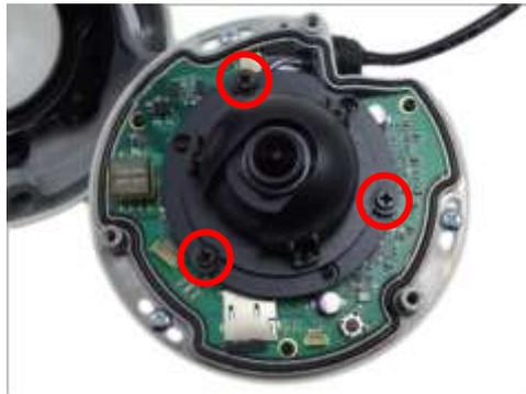
3. Turn the lens module to adjust the camera pan position.
