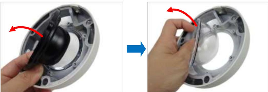
4. Remove the black rubber from the transparent dome cover and place the black rubber to the replacement dome cover.
