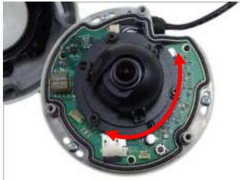
4. Tighten the three (3) screws to fix the pan position.
