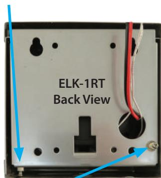
Detects when unit has been removed from the wall
