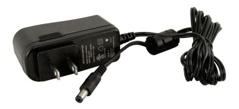
The ELK-P1216 is a general purpose 12 Volts D.C. Switching Plug-In Power Supply. It is ideal for alarm, access control, and CCTV applications requiring up to 1.5 Amps. The power pack plugs into 100 to 120 volts A.C., and supplies regulated 12 volts D.C. to a standard 2.1mm power plug.
