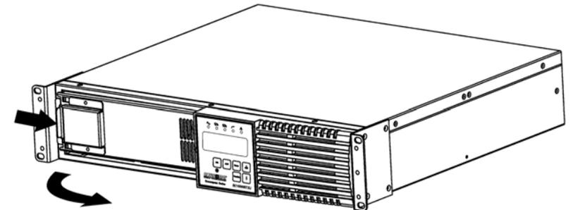
8. Press down to unlock the battery connector holder (FIG. 3).
