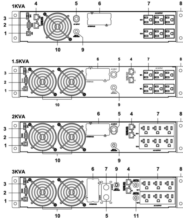
1. The USB Communications Port is for UPS monitoring and control.
