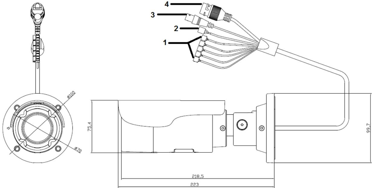
**Figure 31 3MP (IFS03B1ONWIT) and 8MP Cameras dimensions (mm) and pictorial index**
