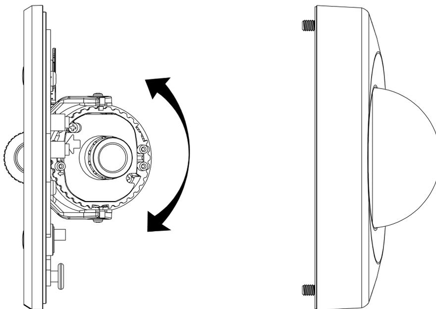
**Figure 58 Adjusting the position of the camera**
