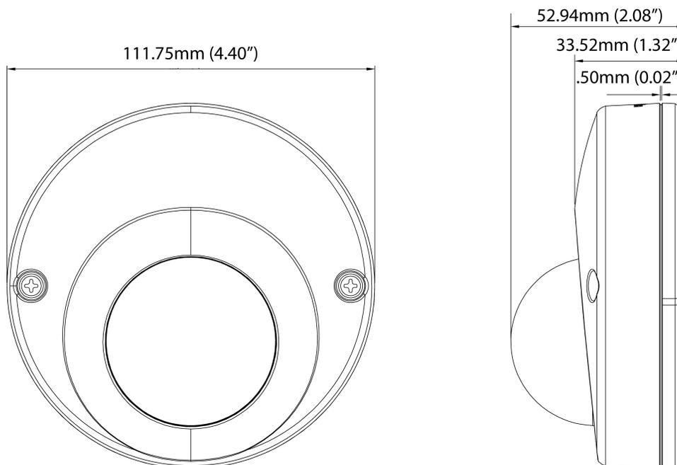
**Figure 50 Physical dimensions of the Compact Mini Dome camera (mm)**
