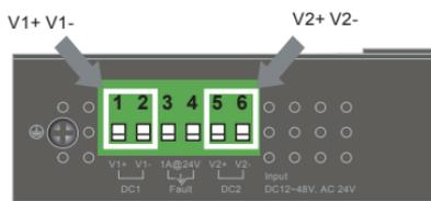
2. Tighten the wire-clamp screws for preventing the wires from loosening.
