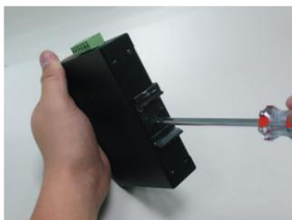
**Step 2:** Lightly insert the DIN rail into the track.
