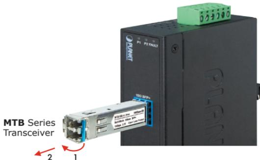
Figure 3-2: Pulling Out from the Transceiver
