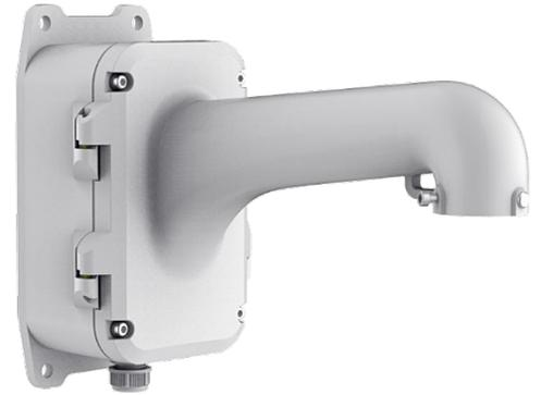
The bracket should be installed on a flat wall. The wall must be capable of supporting over three times the total weight of the speed dome and the bracket. The maximum load capacity of the bracket is 22 lbs (10 kg).
