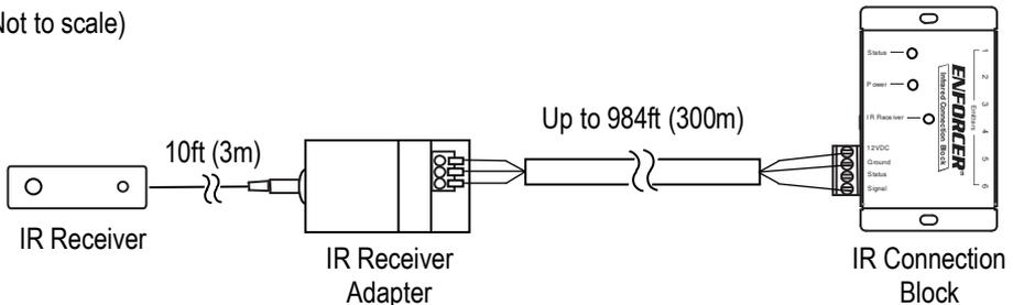
**NOTE:** The "Status" input on the IR connection block is not used when utilizing the IR Receiver Adapter.
