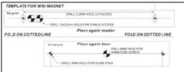
2. Close the door. Find a mounting location on the door frame near the upper free-moving corner of the door, or as close as possible to the upper corner of the door frame opposite the hinges.
