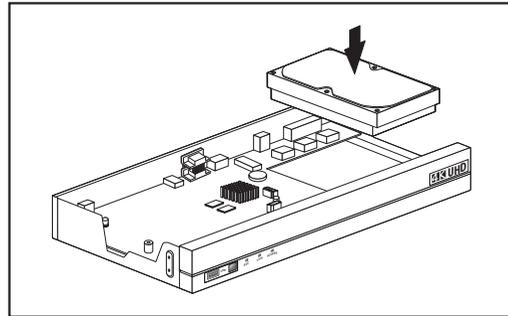
3. Using the screws, fix the HDD to the bottom of the set.
