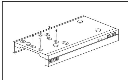
4. Check for any problems in the connection terminal and the wiring in the product, close the cover and fix it with screws.
