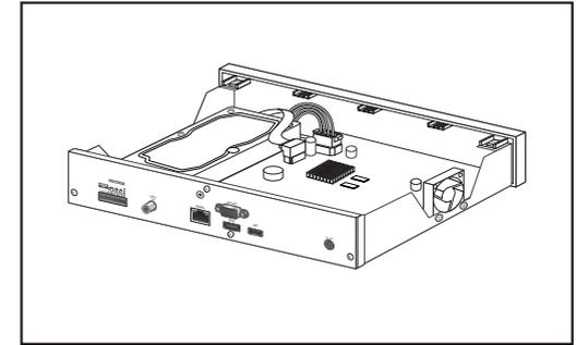
5. Close the cover, and tighten a setscrew in the back.
