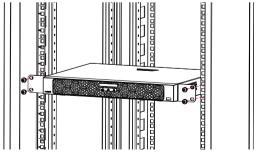
4. Insert the screws into the holes and tighten the screws using a screwdriver.
