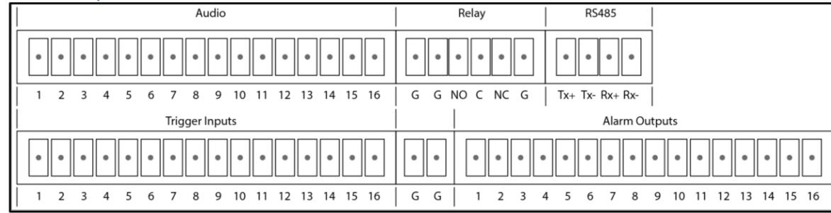
Figure 3: Z-Series 4U Hybrid System auxiliary connections
