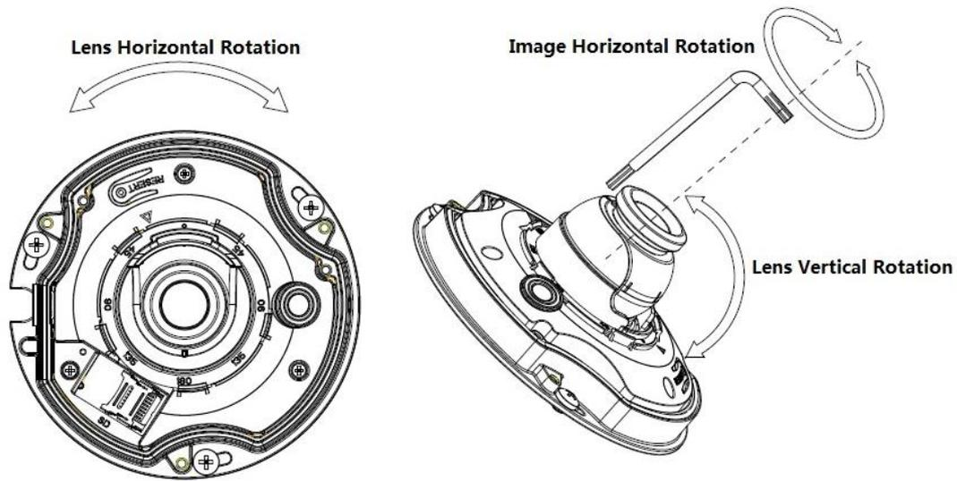
1. Loosen, but do not remove the set screws on either side of the bracket that holds the camera.
