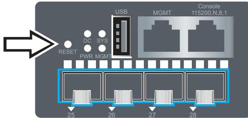
**Figure 6-4:** SGS-6341-16S8C4XR Reset Button
