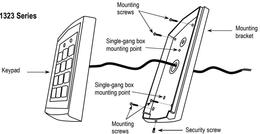
1. Find a suitable location to mount the keypad. Do not install where it will be too high or too low for most users to operate the keypad.
