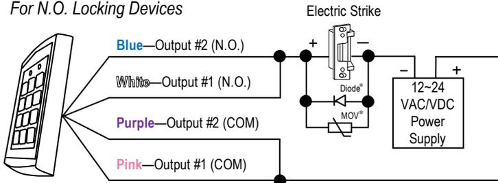
\* Connect included diode and metal oxide varistor (MOV) as close as possible and in parallel with an electric strike. This absorbs possible electromagnetic interference to prevent operation of the strike from damaging the keypad. Do not connect diode or MOV when using electromagnetic locks.
