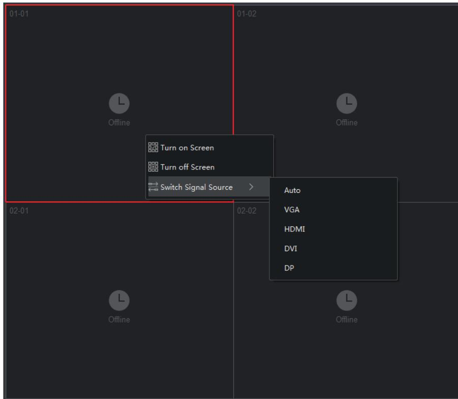
**Figure 4-7 Switch Signal Sources by Right-click**
