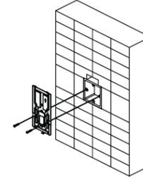
4 Align the device with the mounting plate, and secure the device on the mounting plate with 1 supplied screw (SC-KM3X6-T10-SUSS).
