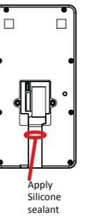
2 Secure the mounting plate on the gang box with two supplied screws (SC-KA4X22).
