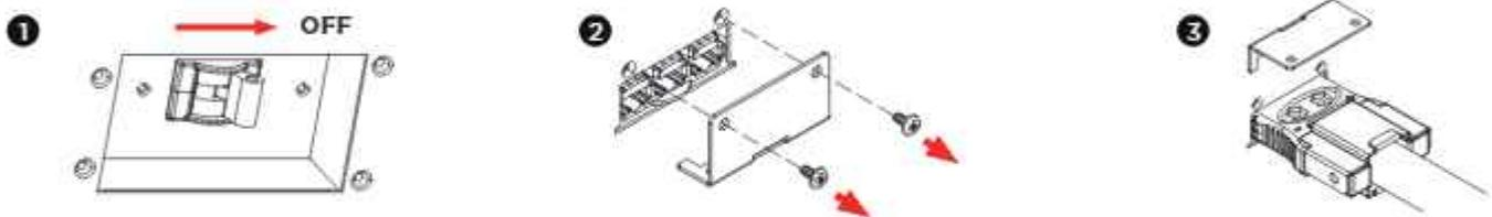
**Step 4:** Rotate the battery cable retention bracket and tighten the two screws to fix battery cable.
