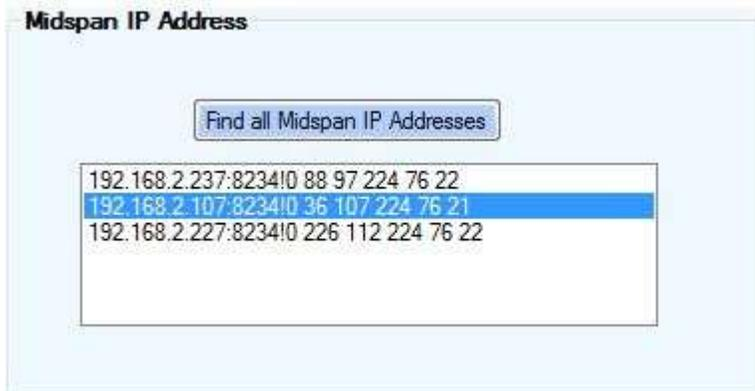
**Step 3 – Program Midspan to operate on your network.** Selecting the Midspan to be programmed in step 2 will place the IP Address into the box labeled “Current IP Address”. If changing the Midspan IP Address is necessary, input the new values for the IP Address, Default Gateway, and Subnet Mask. Then, press the “Program New IP Address”. The example below shows the IP Address being changed from 192.168.2.107 to 192.168.2.117.
