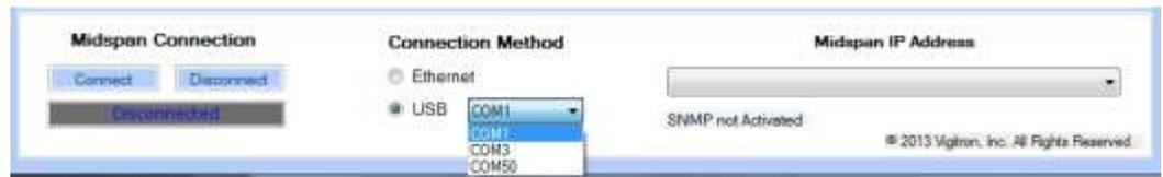
If you are not sure which Com port to select, you can go to the “Device Manager” window of your computer. Click the “Ports” icon and a list of ports will be displayed along with a brief description. The following example shows COM 50 as being a USB serial port. The Midspan is connected to this port. Now you can go back and select the appropriate USB port to use to connect to the Midspan. On the lower portion of the GUI, be sure that the USB button to the left of port selection is clicked.
