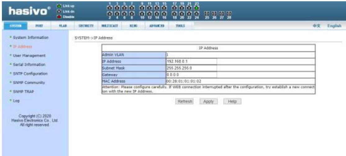
Figure 6 IP address configuration page
