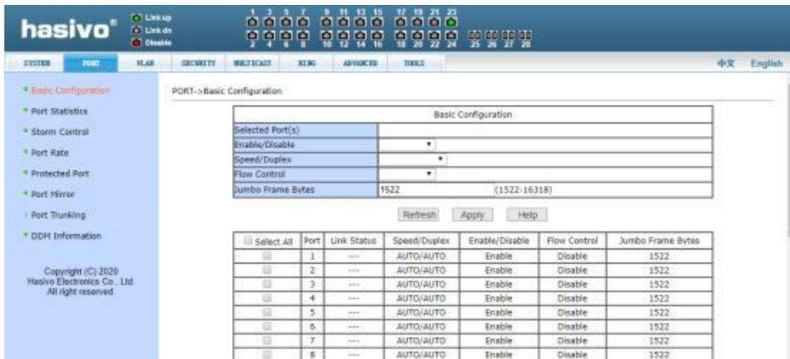
Figure 11 port configuration and port display page
