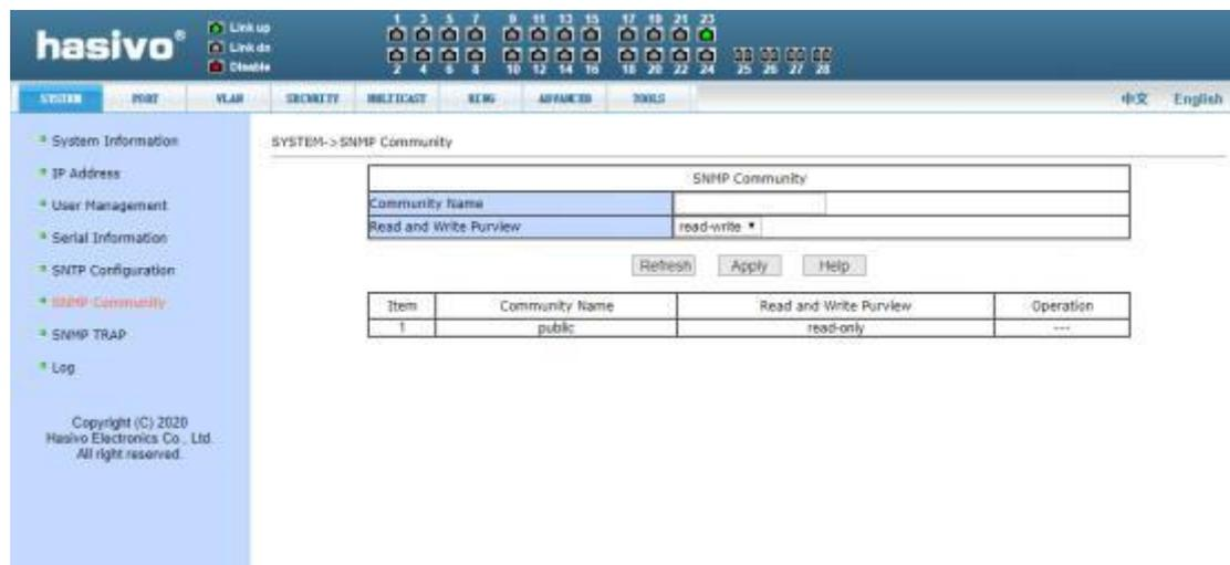
Figure 8 SNMP common configuration page
