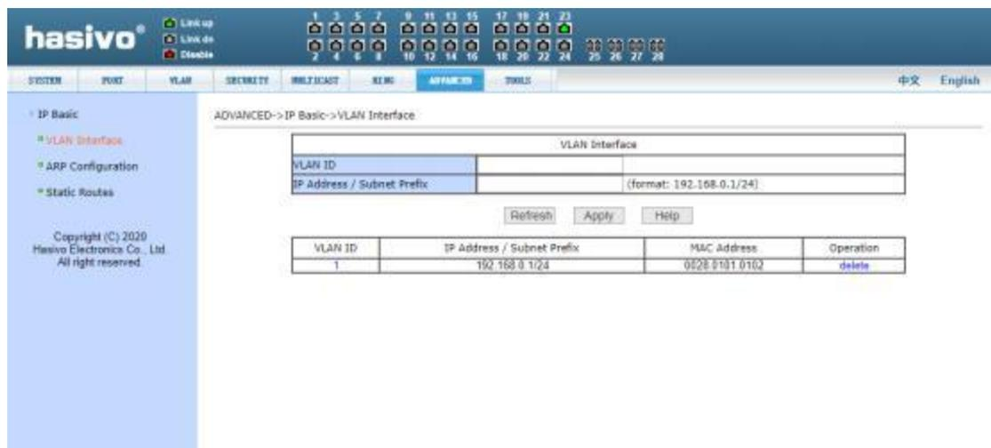
Figure 42 VLAN interface configuration page
