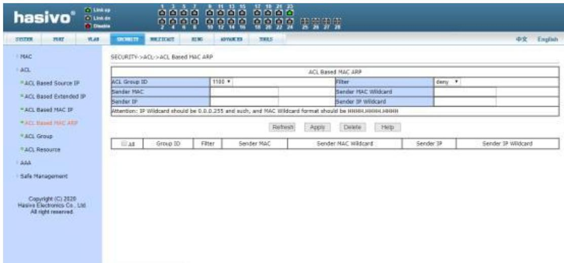
When the user configures the rules, both the sending MAC address and the sending IP address should have address matching bits. The rules can match the set of MAC address and IP address. For example, if the rule matches the IP address range 192.168.0.0 to 192.168.0.255, the IP address can be 192.168.0.1 and its mask is 0.0.0.255.
