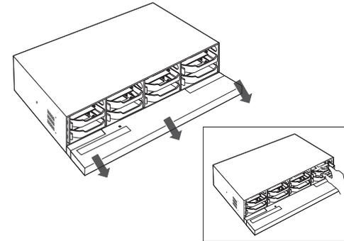
**2** After inserting one side, push and insert the other side slightly
