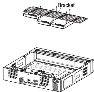
**4** Connect the cable to the HDD by matching the HDD SATA/power cable number to the HDD position number on the bracket.
