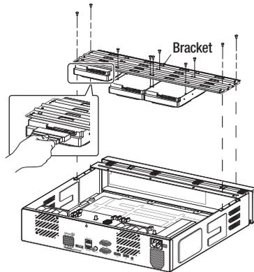
**5** Mount the bracket on which an additional HDD is mounted on the NVR, secure it with screws and connect the SATA/power cable to the connector on the main board by matching the number.
