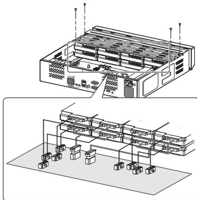
**6** Check for any problems in the connection terminal and the wiring in the product, close the cover and fix it with screws.
