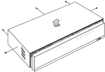
**2** Remove the screws on the left/right side (4 screws) and remove the bracket.
