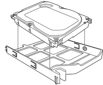
**3** Align and push a bracket in the direction of the board
