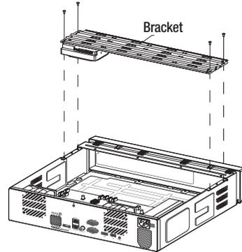
**3** Mount HDDs to the bracket and fix it with screws.
