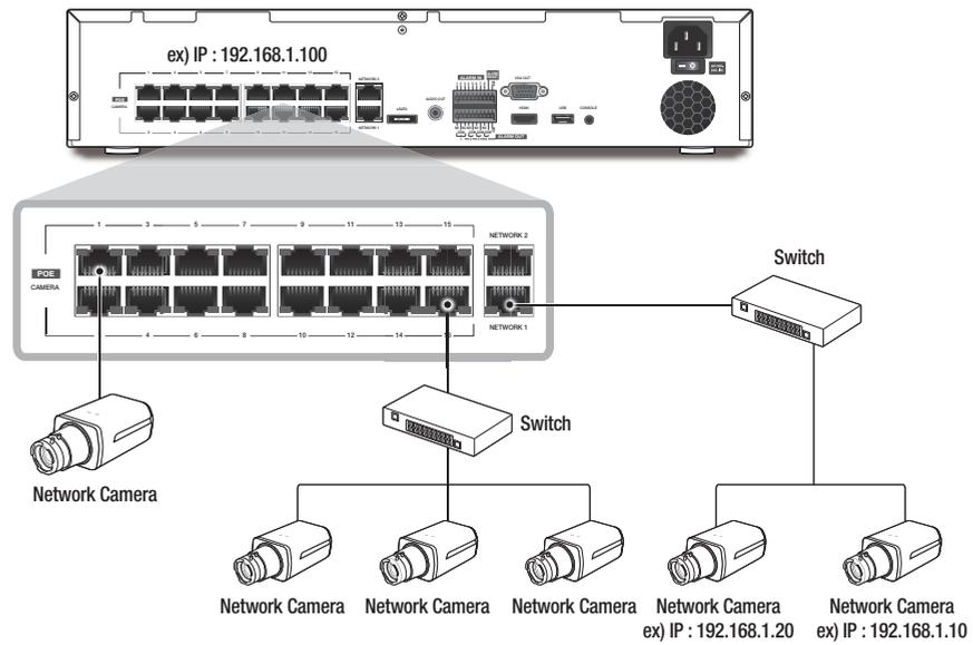
A switch can be used for connection
