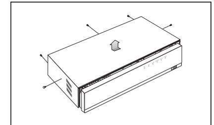
2. Remove the screws on the left/right side (4 screws) and remove the bracket.
