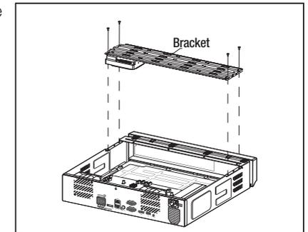
3. Mount an HDD to the bracket and fix it with screws.
