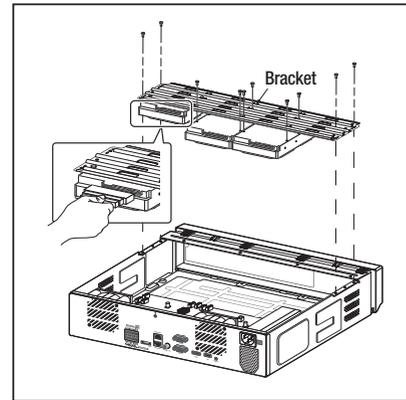
5. Mount the bracket on which an additional HDD is mounted on the NVR, secure it with screws and connect the SATA/power cable to the connector on the main board by matching the number.
