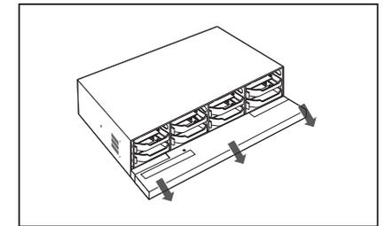
2. Push the latch to the right and remove the HDD bracket.
