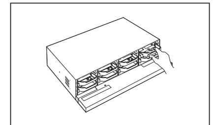
3. Align and insert HDD into the bracket home. After inserting one side, push and insert the other side slightly.
