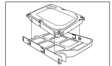
4. Align the bracket with the HDD installed with the enclosure latch, and push the bracket in the direction of the board.
