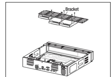
4. Connect the cable to the HDD by matching the HDD SATA/power cable number to the HDD position number on the bracket.
