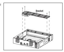
3. Mount an HDD to the bracket and fix it with screws.
