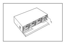
**3.** Align and insert HDD into the bracket home. After inserting one side, push and insert the other side slightly.
