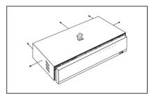
2. Remove the screws on the left/right side (4 screws) and remove the bracket.
