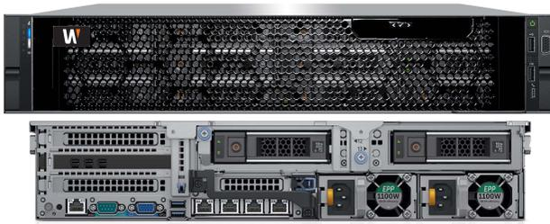
The WRR-P-S202x1 series offers an affordable and reliable 2U rackmount solution for any entry level deployment. Up to 144TB (Linux) / 224TB (Windows) of raw video-optimized storage is provided by 24/7 duty cycle SATA drives.
