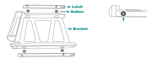
Step2: Get a compatible hard disk. With the PCB side facing down and the hard disk's connector facing the outside. Then, place the hard disk in the HDD tray and insert the latches.
