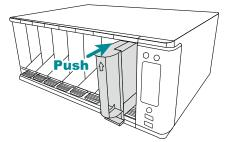
Step5: Replace the front cover removed in Step3 back to the recorder.
