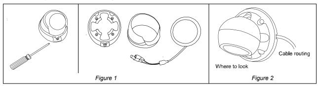
Step3: Drill 4 holes and screw the base to the wall (or ceiling).
