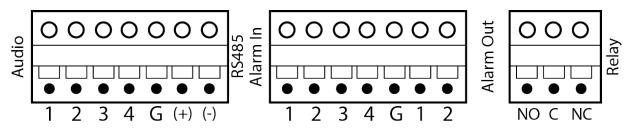
Figure 4: ELP-Series Hybrid System auxiliary connections
