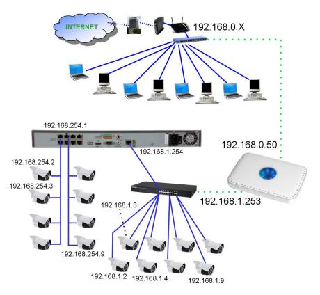
Since routers also function as firewalls, we need to make the NVR accessible from the home/office LAN/WAN side. One way to do this is to indicate the IP address of the NVR (192.168.1.254) as being in the "DMZ" for the
