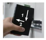
**Step 4:** Lightly pull out the lower DIN-rail bracket first and lift it up to remove it from the track.
