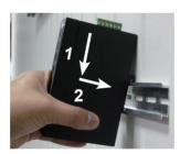
Step 2: Get the lower DIN-rail bracket snapped into the track.
